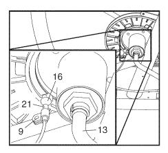
M5 x 12mm Screw (9). Slide the Reed Switch slightly closer to or away from the Magnet, and then retighten the Screw. Turn the Crank for a moment. Repeat until the console displays correct feedback.
